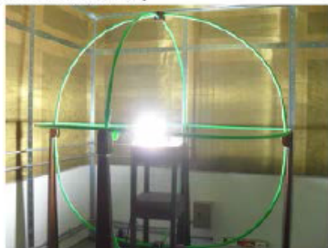
Radiated electromagnetic disturbance - Front View(30 MHz - 503 MHz)
